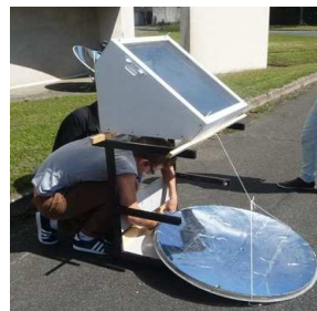
Light reflexion by a parabola – Breaking of the glass result in a concentration of energy
