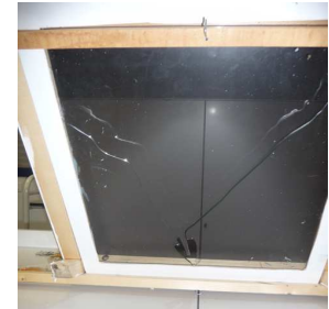
Light reflexion by a parabola – Breaking of the glass result in a concentration of energy
