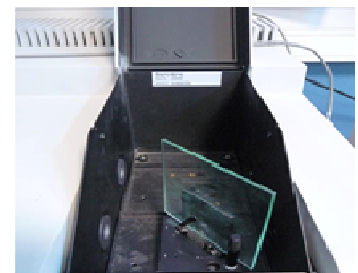
Interior view of a Spectrophotometer with a 45^\circ tilted glass
