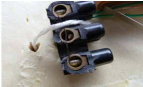
Doc. 8a : First installation of the resistive wire
