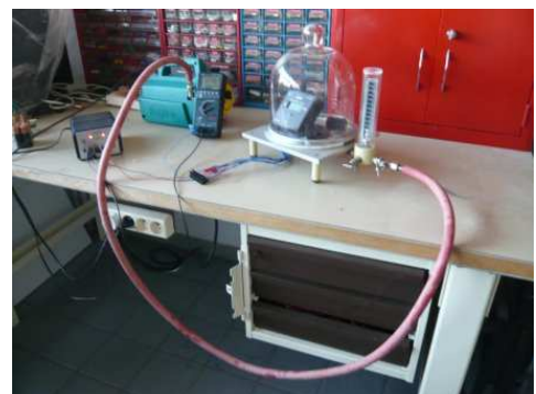
Doc. 3b: Pressure sensor calibration vacuum pump
