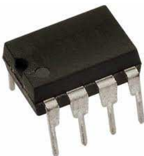
Doc. 5a: Photography of the operational amplifier
